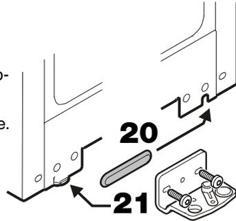
25. Suspend top door on the middle hinge pin and close.
