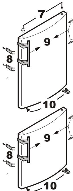
18. Transfer the hinge component on the hinge bracket to the opposite side.
