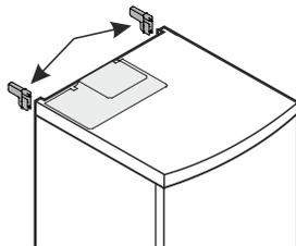
The appliance is fully operational even if the spacers are not used. It does, however, have a slightly higher energy consumption.
