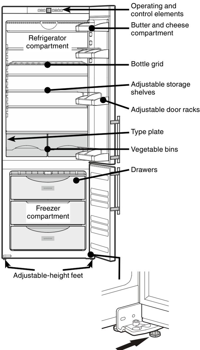
Extend the adjustable foot at the hinge until it rests on the floor and then make a further 90° turn.
