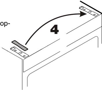
14. Remove hinge bushing, turn through 180° and re-fit.
