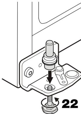
26. Insert hinge bracket and screw into place.
