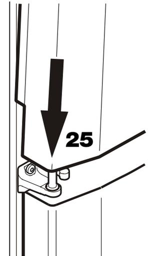
22. Tilt appliance slightly backwards, insert pin and attach using the adjustable foot.
