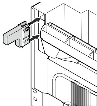
Fit the spacers to the back of the appliance on the left and right at the top.
